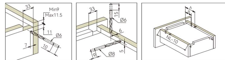
抽屉尺寸和钻孔(mm) Drawer size and drilling
